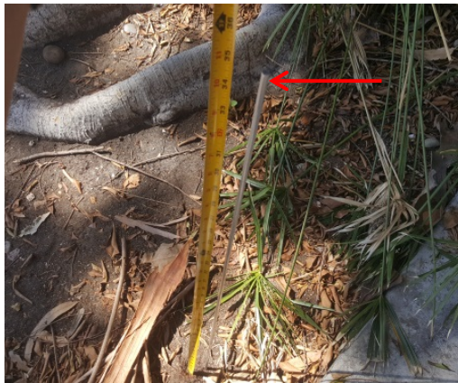
36 Inch Probe Before Insertion
