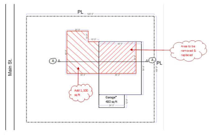
New construction - Condition 1a: More that 50% of the roof framing is removed.
