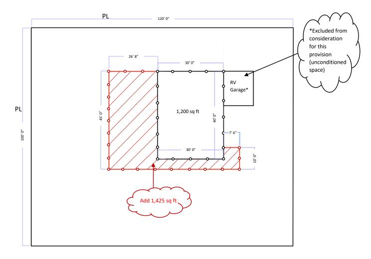
New construction - Condition 1b: More than 50% of the exterior bearing walls (or columns, where there are no walls) are removed.
