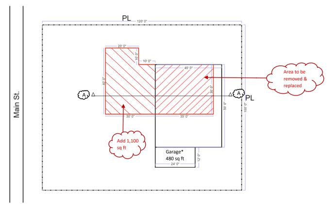
New construction - Condition 1a: More that 50% of the roof framing is removed.
