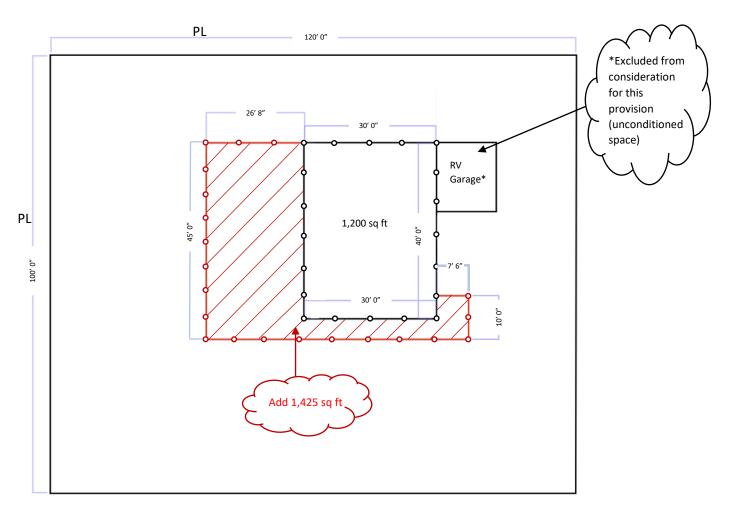
New construction - Condition 1b: More than 50% of the exterior bearing walls (or columns, where there are no walls) are removed. Over 50% of existing exterior columns are impacted by the renovation
