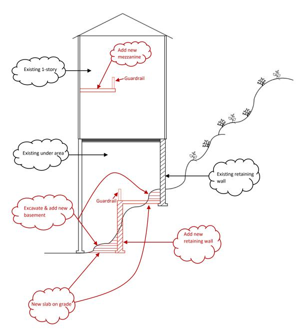
If addition of the mezzanine and the basement result in doubling the volume of the conditioned space, then Condition 2 is met. Albeit for the purpose of the CBC, mezzanine and basement may be exempt from floor area calculations.
