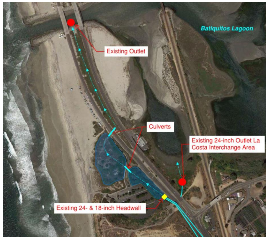
Figure 2: L101 Area Existing Storm Drain Outfalls
