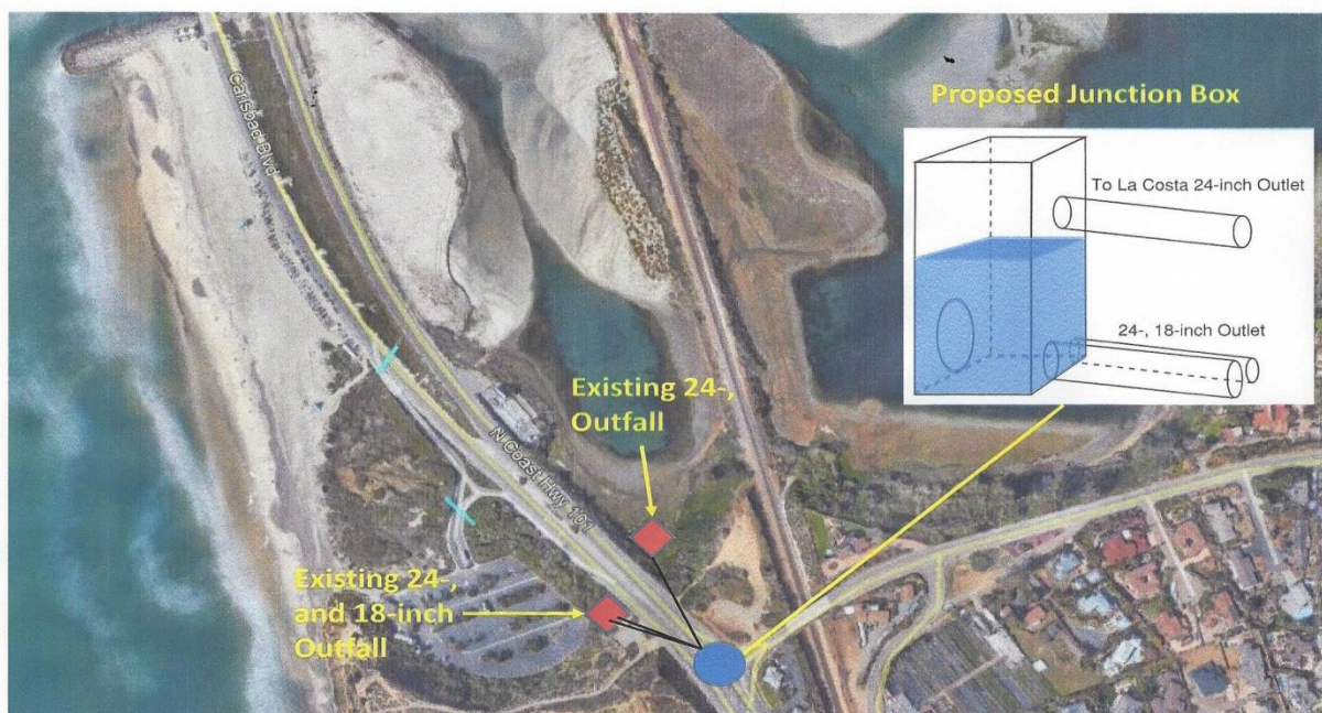
Figure 1. Existing Batiquitos Lagoon stormwater outfalls and proposed junction box.
