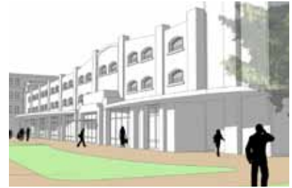
Design floor to floor heights to establish a sense of scale and respond to that of the surrounding context.
