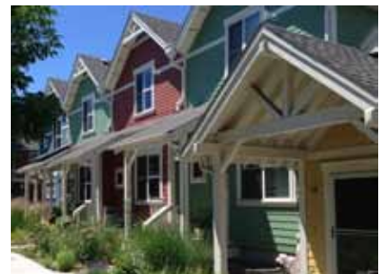
Larger, new development should vary the facades to appear to be smaller, individual structures.
