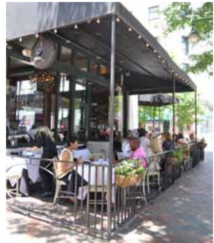
A railing, detectable barrier, or similar edge treatment can be used to define the perimeter of a permanent outdoor dining area.
