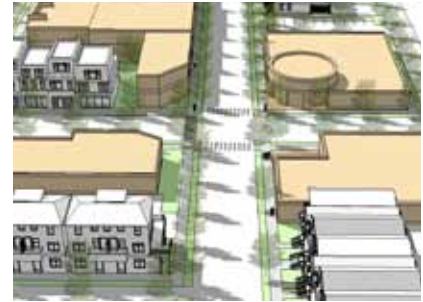
Maintain a defined street edge. A new building should help define and enclose the streets.
