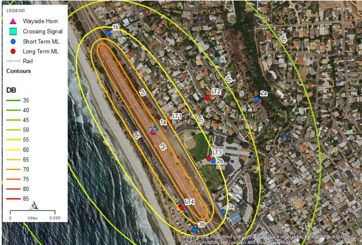
Figure 4-19. Locomotive Horn Noise Contours
