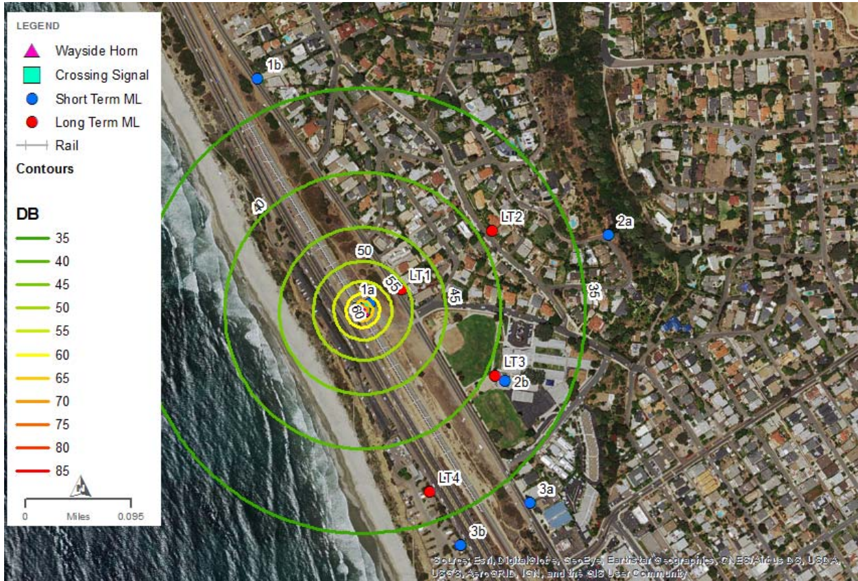
Figure 4-18. Option 3 Wayside Horn Noise Contours
