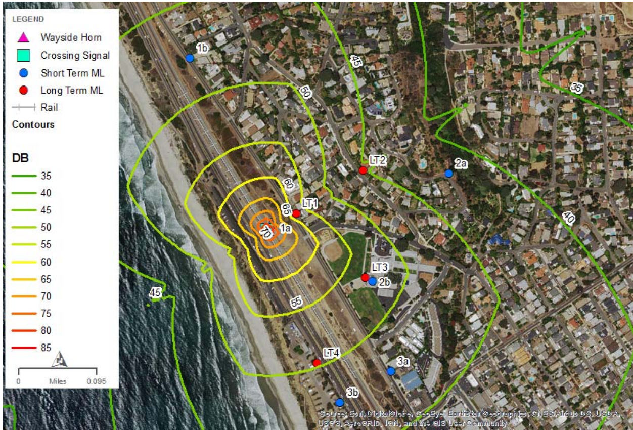
Figure 4-17. Option 2 Wayside Horn Noise Contours
