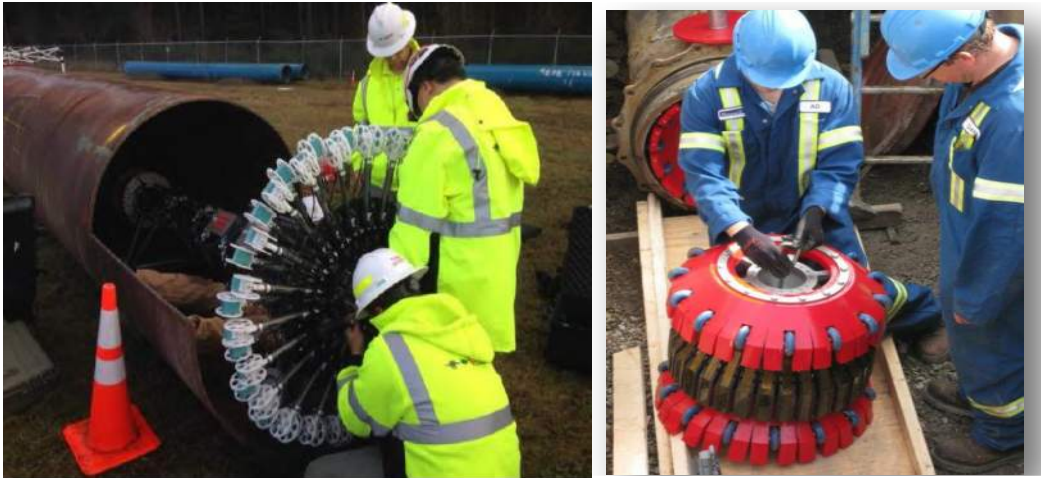
Figure 4. Example of In-Pipe Electromagnetic Technology
